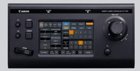
Canon's RC-IP100 Remote Camera Controller provides control for a Canon camera through the serial port. Additionally, up to 99 supported Canon cameras can be operated via IP control. The controller is equipped with a 7" interactive touch screen and a joystick in order to pan, tilt, zoom and change camera function settings remotely. The smooth precision of the joystick allows operators to capture on-air movements with confidence.
