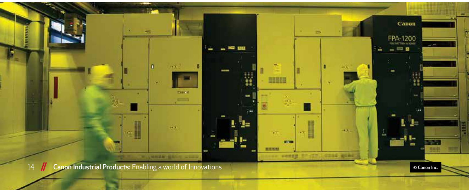
Canon Jet & Flash Imprint Lithography (J-FIL) Nanoimprint Process
